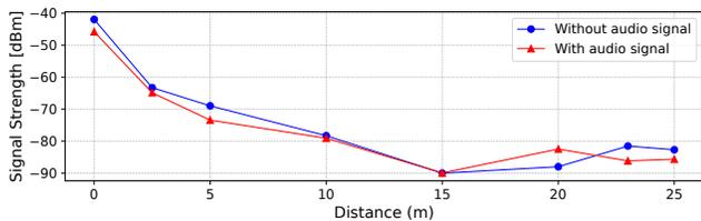
Figure 9: *TUNNELRADIO* maximum range. We observed that the signal strength of the received signal from the tunnel diode transmitter falls below the sensitivity levels of the receiver at a distance of 23 metres. This represents the range achieved in our experiments presented in this work.
