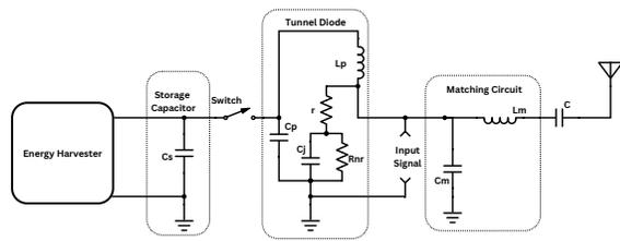
Figure 4: Schematic of the TUNNELRADIO. The tunnel diode is coupled to a resonant circuit to generate oscillations in the FM band. The properties of the resonant circuit dictate the TDO frequency. Using the SoM and self-modulation property, the carrier signal is modulated with a baseband or an audio signal.
