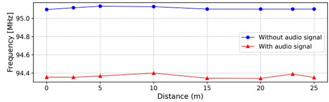
Figure 10: *Stability of the resonant frequency of the TDO.* The frequency remains stable and exhibit minimal drift during the course of the experiment.
