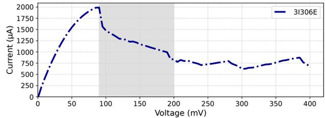
**Figure 3: I-V characteristics of 3I-306E Ga-As tunnel diode. The tunnel diode exhibits a region of negative resistance at low voltages and currents. The overall power consumption of the diode remains well below 150 microwatts, which is sufficiently low to be powered by ambient energy sources**
