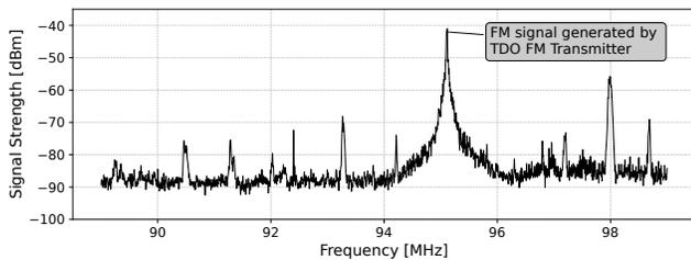
Figure 5: Unmodulated TUNNELRADIO spectrum. We observe a carrier signal generated from the TUNNELRADIO at a center frequency of 95.1 MHz. We also observe FM stations present in the vicinity of TUNNELRADIO transmissions.
