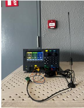
Figure 7: *TUNNELRADIO* setup. It is connected to standard FM antenna
