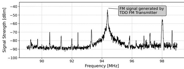
Figure 8: *TUNNELRADIO* transmitter modulated with audio signal. We observe transmission at the frequency of 94.4 MHz. Due to the self-modulating property, the carrier signal is modulated with the audio signal without sidebands.
