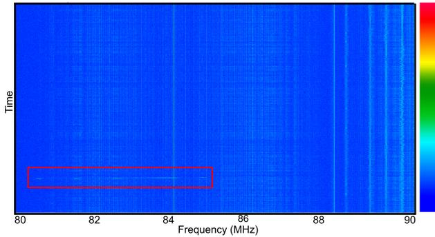
Figure 12: *Operations on harvested energy.* We can power the TUNNELRADIO transmitter on energy harvested from RF signal. Owing to the small size of the capacitor, the transmitter was turned on for short period of time, and can be see through a horizontal line in the waterfall plot. The change in the capacitor voltage leads to change in the resonant frequency.
