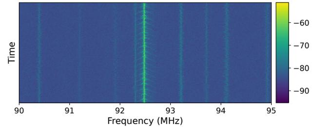
Figure 11: *Modulating TUNNELRADIO with complex baseband signal.* We observe the chirps in the waterfall plot. They are generated as we mix a chirp-modulated baseband with the carrier signal generated from a TDO.
