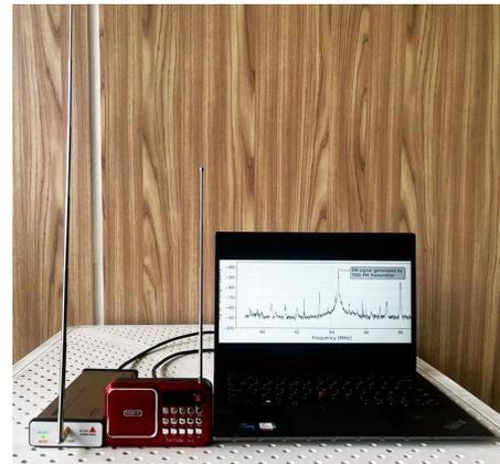
Figure 6: Receiving setup. For receiving broadcasts, we use a COTS radio. To receive complex baseband broadcasts, we use a spectrum analyser.
