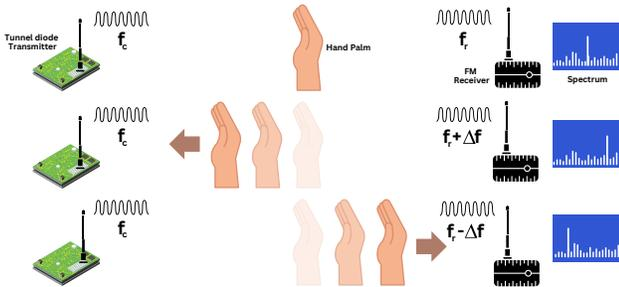
Figure 13: *TUNNELRADIO can also help with sensing.* Macroscopic motion in the vicinity, such as, hand gestures alter the frequency of these emissions. For applications like vital sign monitoring and gesture recognition, these frequency variations can be tracked and analyzed by a COTS FM receiver.
