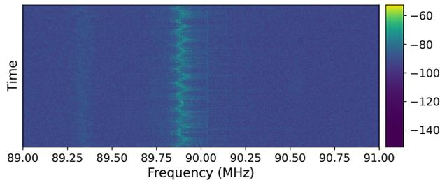
Figure 14: *TUNNELRADIO frequency variations.* We observe deviations in the frequency of the TDO due to hand gestures in the vicinity of the TUNNELRADIO. This is due to the sensitivity of the TDO to the changes in the environment.
