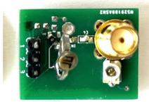
**Figure 2: TUNNELRADIO hardware.** It is designed with a minimal number of components. The dimensions of the board are on the centimeter scale. The small form factor and low power consumption can facilitate usage in WES.
