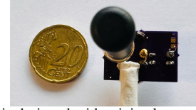
Fig. 2. TunnelSense is designed with minimal components, which allows the platform in its simplest form to be as compact as a coin cell. The simplicity of the circuit and low-power consumption can also enable the realization of the sensor in novel form factors, such as postage stamp sized stickers.
